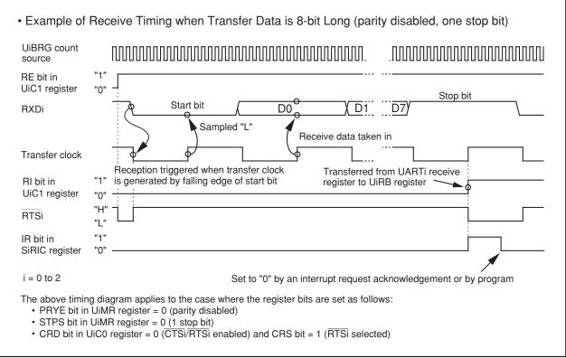
Figure 14.18 Receive Operation
